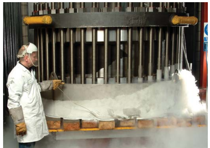
70" 150 lb valve cooling down for cryogenic test.
