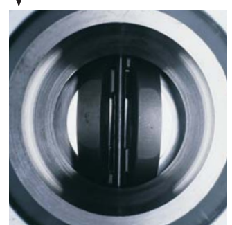
Flow area as viewed through flange on outlet side of valve.
