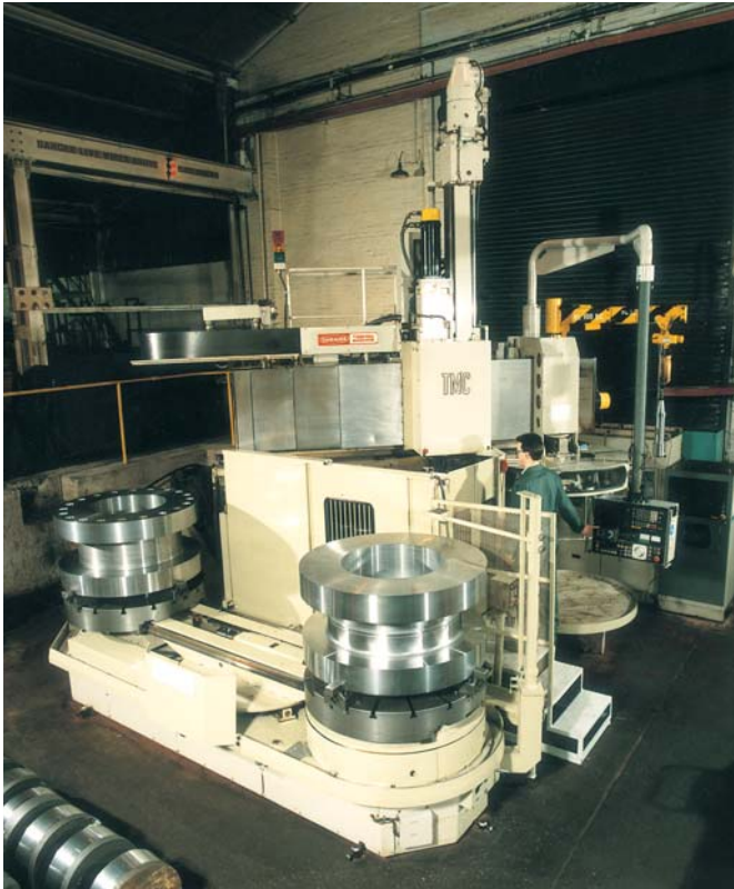
Three station CNC vertical borer with live spindle and tool changer
