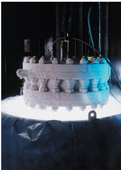
24"ANSI 150lb Check Valve on Cryogenic Test
