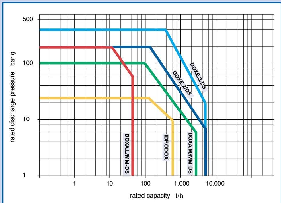
these diagrams give a general overview of available pumps and their performance range and can be used to select the model suitable for your application; for a more accurate selection and in case of particular process requirements, we recommend that you contact either OMG sales offices or your local OMG representative
